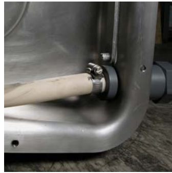
Slide the hose onto the barbed fitting then tighten the hose clamp over the barbed area. Repeat for the second clamp.
