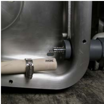
Slide a hose clamp over the end of the hose.
