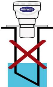
The maximum level (100% of Span) is inside the Blanking Distance
