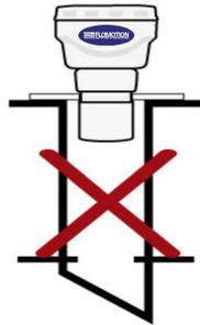
Pipe should be free of obstructions such as weld seams
