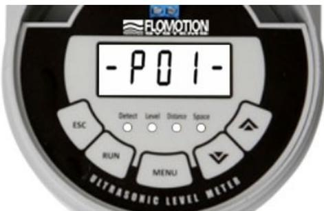
This mode is used to set up the FM1100C or change information already set, this is achieved by using the 5 push buttons located either side of the display.
