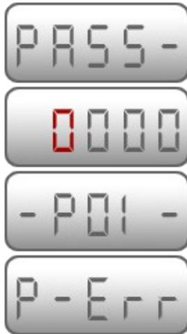
1. If the password is not "0", the "pass" shows on the display.
