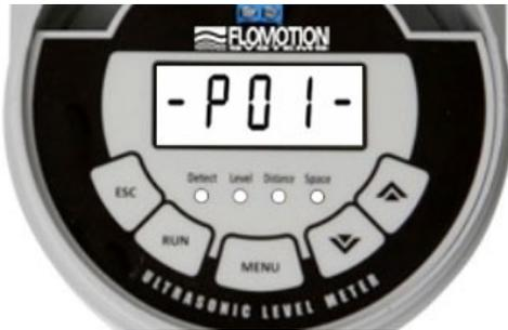
This mode is used to set up the LT330 or change information already set, this is achieved by using the 5 push buttons located either side of the display.
