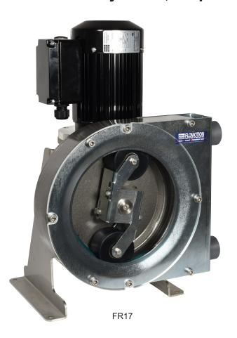
The FR17 is a two roller peristaltic pump designed to handle abrasive slurries, viscous fluids, and aggressive chemicals that are normally difficult to pump with other types of positive displacement technologies. The FR17 is an ideal choice for metering, batching and transfer applications. Peristaltic pumps are becoming the standard for hard to handle fluids such as Sodium Hypochlorite that off-gas and vapor-lock diaphragm pumps.
