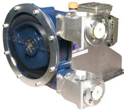
The FS15 Series peristaltic pump is a lobe design on a rotating wheel successively compressing a reinforced rubber hose. The motion of the lobes compresses the rubber against the pump housing creating continuous suction at the inlet of the pump and pushing the fluid to the outlet of the pump.
