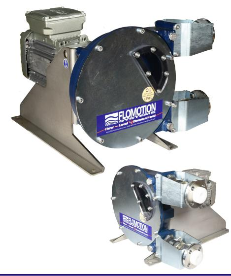
The FS25 Series peristaltic pump is a two-shoe design, 180° apart on a rotating wheel, successively compressing a reinforced rubber hose. The motion of the shoes compresses the rubber against the pump housing creating continuous suction at the inlet of the pump and pushing the fluid to the outlet of the pump.
