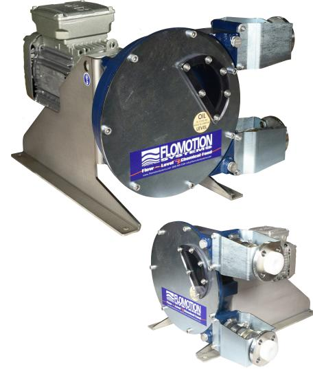
The FS32 Series peristaltic pump is a two-shoe design, 180° apart on a rotating wheel, successively compressing a reinforced rubber hose. The motion of the shoes compresses the rubber against the pump housing creating continuous suction at the inlet of the pump and pushing the fluid to the outlet of the pump.
