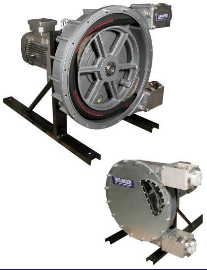
The FS40 Series peristaltic pump is a two-shoe design, 180° apart on a rotating wheel, successively compressing a reinforced rubber hose. The motion of the shoes compresses the rubber against the pump housing creating continuous suction at the inlet of the pump and pushing the fluid to the outlet of the pump.
