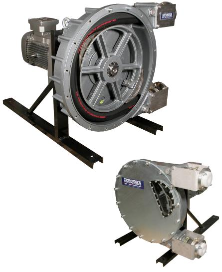
The FS50 Series peristaltic pump is a two-shoe design, 180° apart on a rotating wheel, successively compressing a reinforced rubber hose. The motion of the shoes compresses the rubber against the pump housing creating continuous suction at the inlet of the pump and pushing the fluid to the outlet of the pump.
