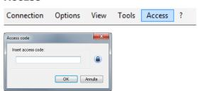
□ Access: Opens the window where you can enter the access code provided by the manufacturer that allows you to activate the various functions the converter. Access code or code of level rule therefore the presence or absence (from access level 2 and above) of a specified number of functions in the function list. To launch this window quickly click command Ctrl + A.
