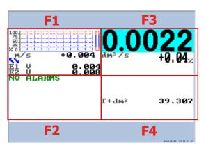
The virtual display is divided into 4 sections. In each of them there are the different parameters set in the converter drive.
