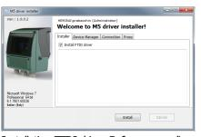
Installation FTDI driver. Before proceeding with the installation dick "Install FTDI drivers"
