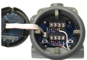
The PD6720 is a NEMA4X field mounted, loop-powered meter fully featured for demanding applications in wet or dirty environments.
