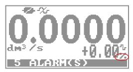
Symbol that is activated when there is a dynamic variation of the flow measurement. It indicates that the measurement shown in the display is stabilizing.
