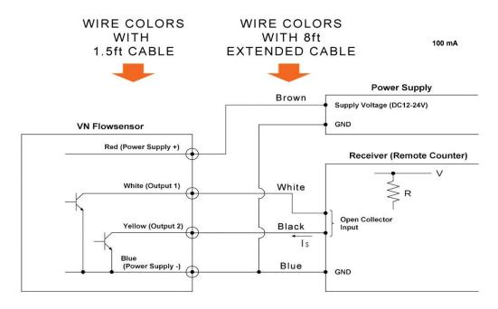
V (Pull-up voltage) Is (Absorbing current of output) =  $\frac{}{\text{R (Pull-up resistance)}} \leq 20 \text{mA}$
