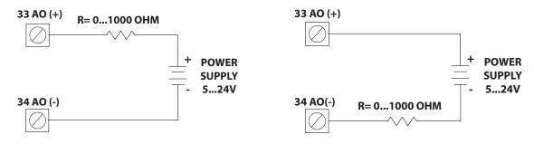
The maximum load value for the PASSIVE connection depends on the supply voltage supplied. The maximum 1000 ohms of load are guaranteed only with supply voltage> = 25V.
