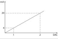
The diagram shows how the DAC4-20mA parameters are setup. The DAC1 value corresponds to 4 mA corresponding to a zero flow rate, while the value of 20mA corresponds to a 100% of the flow rate.
