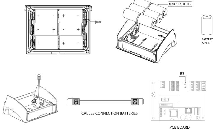
Connections to B1 and B2 are not used and no other batteries must be connected to the instrument.
