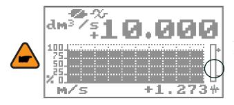
This symbol appears (red color on the virtual display) only when the overall noise is over 2.5% of flow rate.
