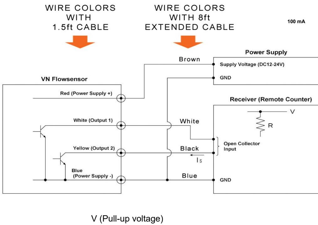
$$I_s \text{ (Absorbing current of output)} = \frac{V}{R \text{ (Pull-up resistance)}} \leq 20 \text{ mA}$$
